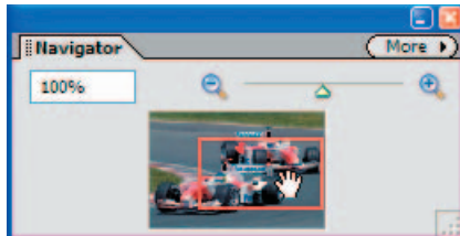
Figure 2.19 The marquee feature available in Navigator allows for convenient review of various image areas by dragging the red box to elements that you want to scrutinize.
